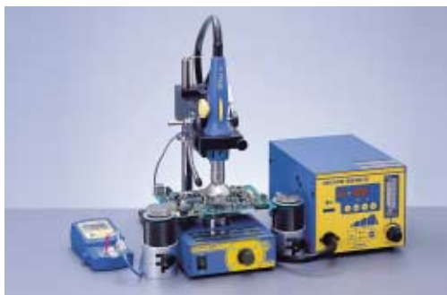
Setting example HAKKO FR-803B, HAKKO FR-830, Rework Fixture, Omnivise
